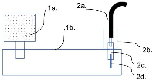
**Figure 8: EX-1;** 800W 5.8 GHz magnetron AIR-COOLED (1a), Universal magnetron launcher and WR159 transition waveguide to N-type female connector (UML-TW) (1b.), 2m coaxial cable with N-type male connector to N-type female bulkhead (2a.), N-type female bulkhead (2b.), coupling pin (2c.), direction of thrust of coupling pin (2d.)
