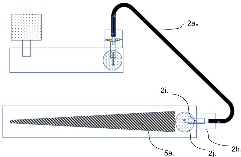
**Figure 11:** EX.1; 2m coaxial cable with N-type male connector to N-type female bulkhead (2a.), N-type female bulkhead (2h.), gravielectric chamber coupling pin (2i.), proposed EM resonance field region (2d.), internal steel rod tapered from 22.3mm diameter to 12mm diameter (5a.)
