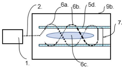
**Figure 12:** RF source (1.), connecting coaxial lead (2.), one solenoid (6a.) ~5 winds forward (image 7), another solenoid (6b.) ~5 winds back (image 7), solenoid winding Perspex tube bulkhead (5d.) attached to 51.7mm ID aluminium pipe structure (9b.), EM destructive-interference field region (6c.), solenoid wind diameter 25.8mm (7.), see images 6-9.
