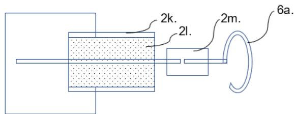
**Figure 15:** male N-type connector (2k., image 17), male N-type connector insulator (2l., image 18), antenna safety plug (2m., image 20), internal solenoid (6a, image 6)
