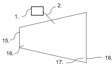
**Figure 17:** Conventional EM thruster; magnetron microwave source (1.), attachment/coaxial cable (2.), smaller diameter end of vacuum chamber cavity (15.), obtuse angle between smaller cavity end and tapered cavity wall (16.), acute angle between larger cavity end and cavity wall (17.), larger diameter end of cavity (18.)
