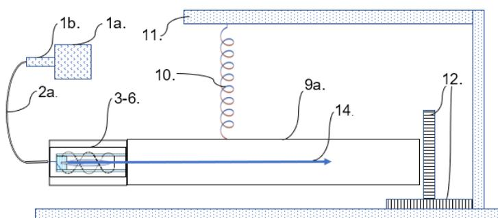
**Figure 14:** 800W 5.8 GHz magnetron AIR-COOLED (1a), Universal magnetron launcher and WR159 transition waveguide to N-type female connector (UML-TW) (1b.), 1m coaxial cable with N-type male connector to N-type female bulkhead (2a.), internal aerial system (3-6.), 74MM ID 1130MM long aluminum cavity tube (9a.), Aluminum tube suspended horizontally from swivel-arm (11.) by spring (10.), measurement rulers to measure movement at the distal end (12.), anticipated direction of thrust/movement (14.)
