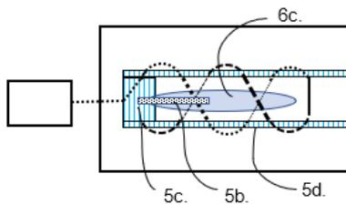
**Figure 13:** Perspex rod bulkhead (5c.) attached to Perspex tube bulkhead (5d.), rod (5b.), see image 8, exposed to EM resonant field (6c.)
