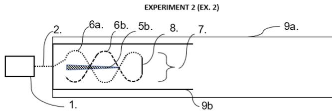
**Figure 4: EX-2;** AC/pulsing power supply for solenoids (1.), connecting coaxial lead (2.), one solenoid (6a.), another solenoid (6b.), solenoid core rod (5b.), solenoid wind diameter (7.), wire joining solenoids at one end (8.), aluminium tube cavity chamber 74MM ID (9a.), inner aluminium tube cavity chamber 51.7MM ID (9b.)
