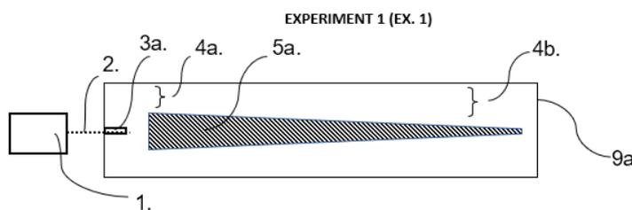
**Figure 3: EX-1;** AC/pulsing power supply for solenoids (1.), connecting coaxial lead (2.), chamber coupling pin (3a.), chamber ideal circumferential distance 25.8mm (4a.), chamber non-ideal circumferential distance ~31mm (4b.), internal steel rod tapered from 22.3mm diameter to 12mm diameter (5a.), aluminium tube cavity chamber 74mm ID (9a.).
