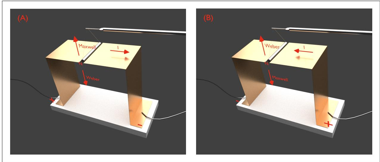
Fig. 6: Experimental setup: capacitor and permanent magnet (north pole directed towards the observer)
