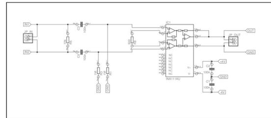
Fig. 8: measuring amplifier
