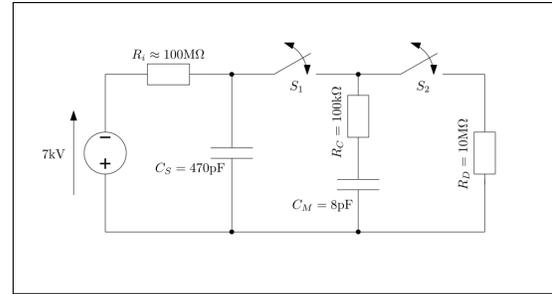
Fig. 7: charging circuit
