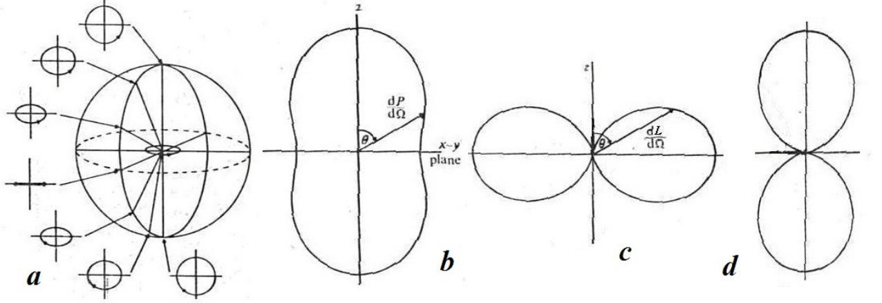
Fig. 2. An electric dipole rotating in the  $x$ - $y$  plane
