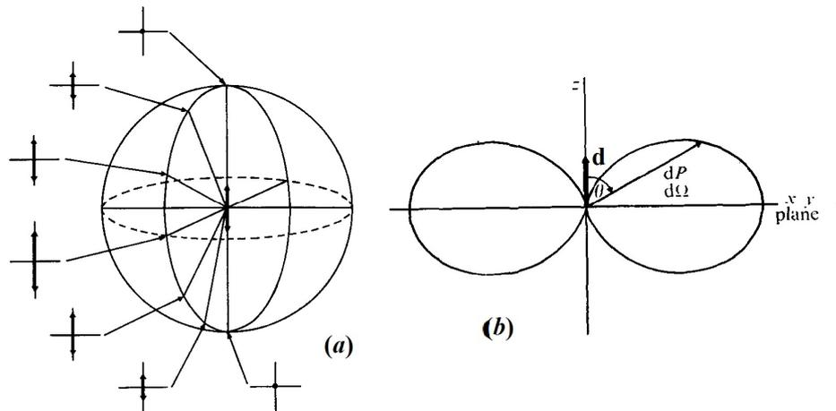
Fig. 1. An electric dipole oscillating parallel to the z-axis.
