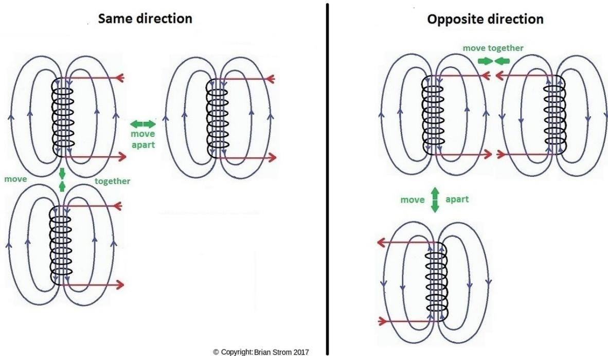
**Figure 11: Summary of interactions between energy fields of coiled-conductors.**
