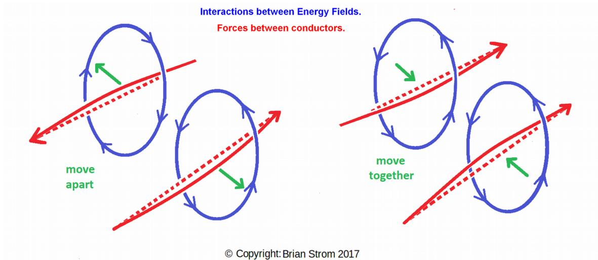
Figure 7: Interaction between Energy Fields around conductors.
