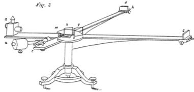
Fig. 7. Michelson's 1881 interferometer<sup>29</sup>.
