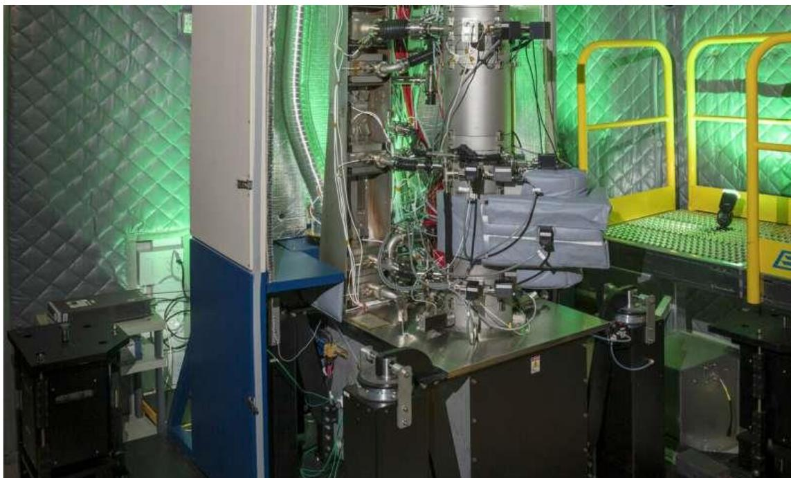
Oak Ridge National Laboratory scientists used a monochromated, aberration-corrected scanning transmission electron microscope, or MAC-STEM, technique that detects the subtle changes in the weight of proteins at the nanoscale--while keeping ...[more](#)"Now, we can track isotopic labels
