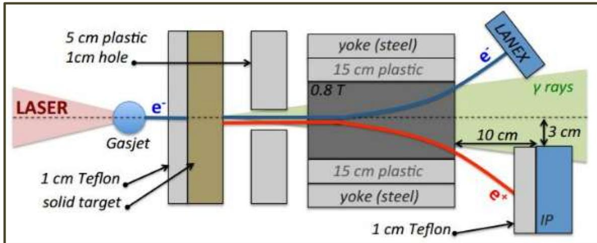
**Figure 24: Laser Generated Electron and Positron Generation Setup**
