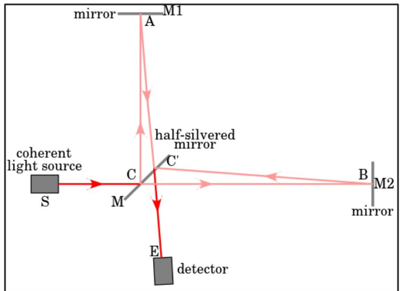
**Figure 46: Michelson Interferometer setup: parallel merged beams**
