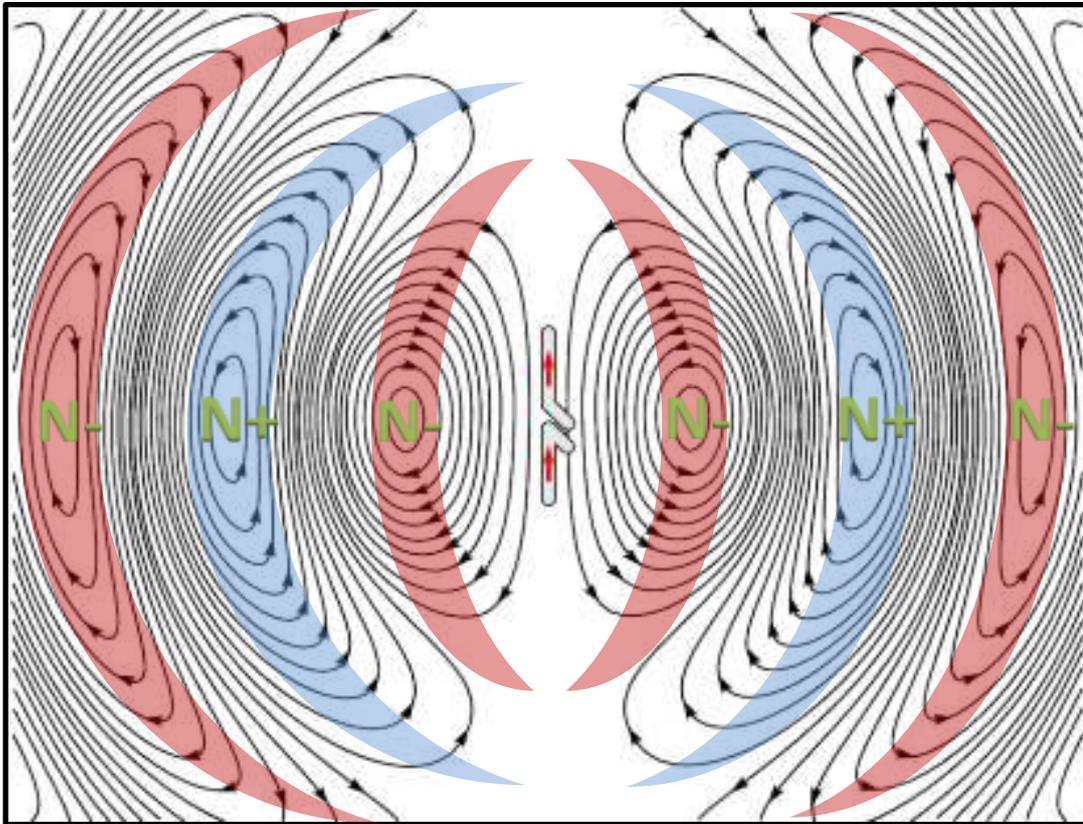
**Figure 45: Electromagnetic Field Patterns for a Dipolar Antenna**
