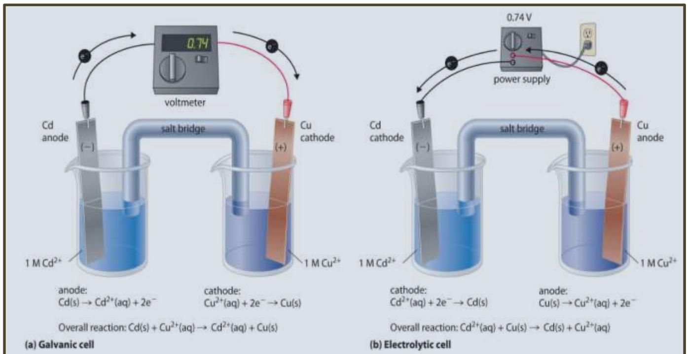
**Figure 53: Galvanic and Electrolytic Cells**
