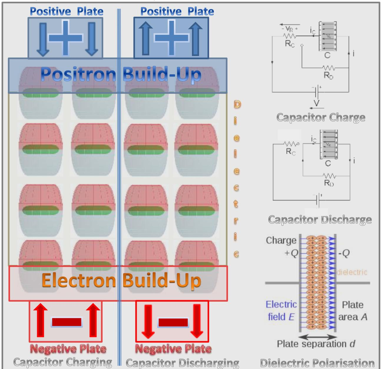
Figure 52: Electric Capacitor Charge and Discharge Phases
