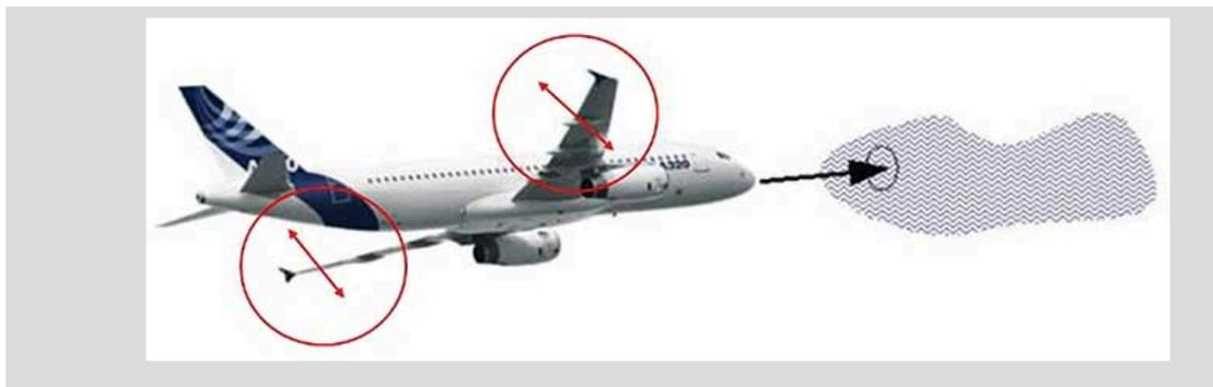
**Figure 4.** Aircraft being equipped with forward-looking lidar are able to counterbalance turbulence and gust influence (lift change, wing loads, accelerations) by deflecting control surfaces. Courtesy of Airbus.
