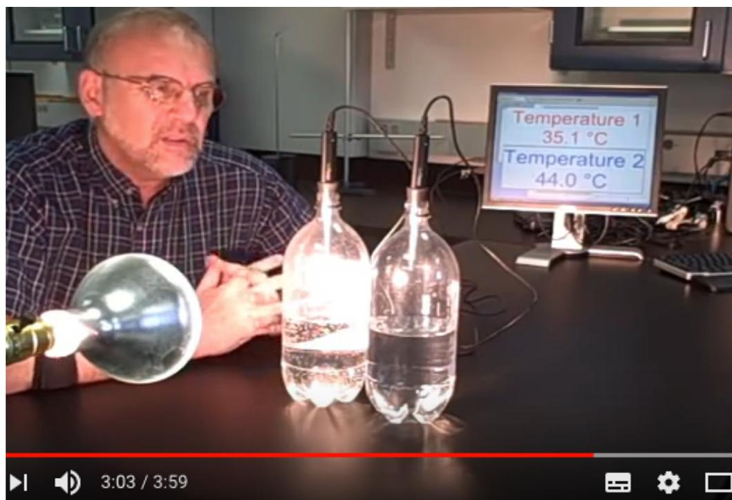
**Figure 46. Greenhouse Gas Bottle Demonstration [69].** Bottles with CO<sub>2</sub> and air are radiated and temperature measured – CO<sub>2</sub> in blue. Is this not an experiment to measure the heat capacities of the respective gases?
