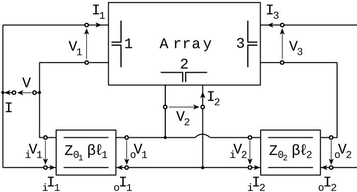
Fig. 7: Equivalent circuit of the 3 dipoles linear array
