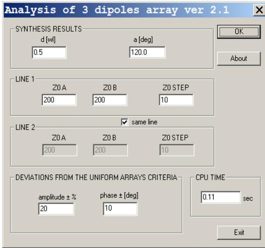
Fig. 14: GUI for Quasi-Uniform Array of  $N = 3$  dipoles
