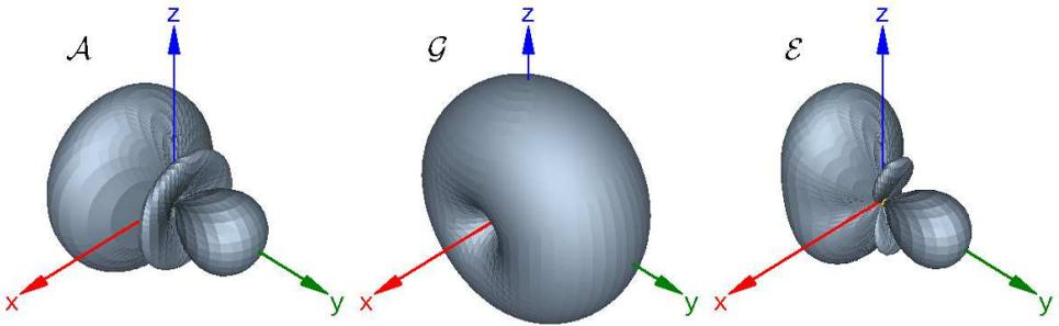
Fig. 24: Multiplication Principle: 3D patterns in dB [5]
