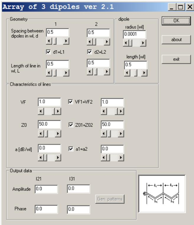
Fig. 8: GUI for the analysis of a linear array
