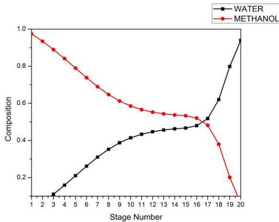
Fig. 4. Variation of composition of methanol and water in liquid phase v/s stage number
