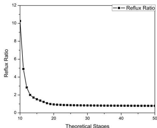
Fig. 3. Reflux ratio v/s Theoretical stages
