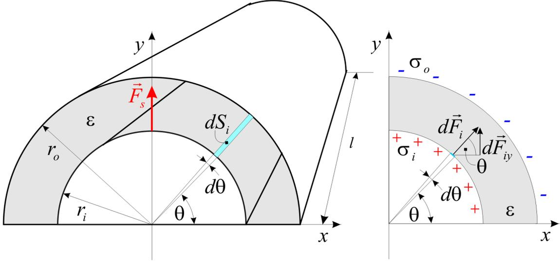
Figure 2: Calculating the  $y$  component of electrostatic pressure forces in the top 180° sector.
