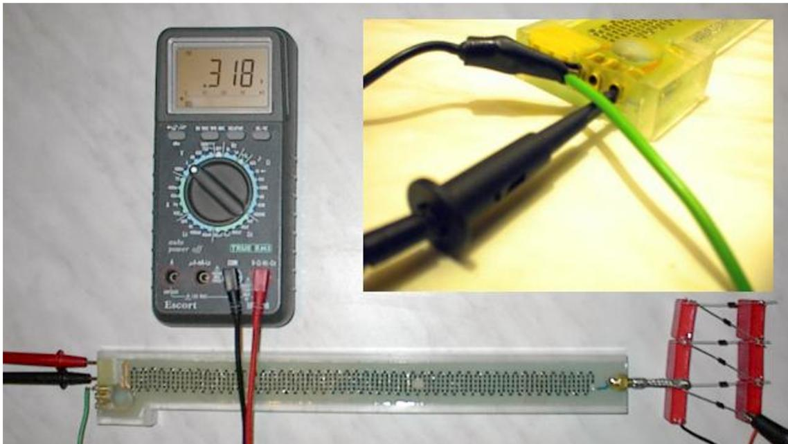
Figure 26: Checking the transfer ratio of the probe (0.318 V is indicated), and an illustration of the oscilloscope's probe being hooked onto the output connector through the screw-holes at the bottom.
