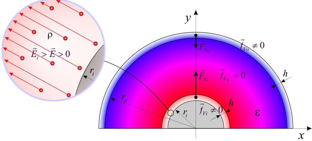
Figure 5: Converting the 2D electrode boundary surface into a 3D layer of thickness  $h$ .
