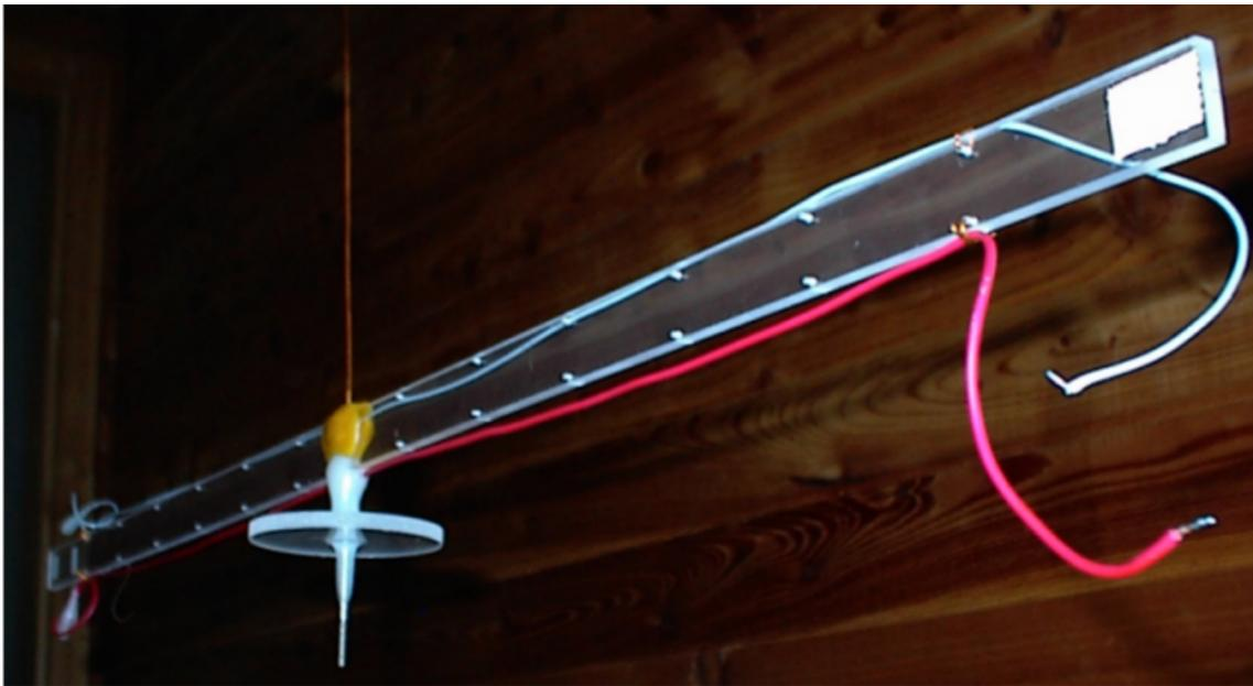
Figure 16: The torsion pendulum with the beam ready for measurements.
