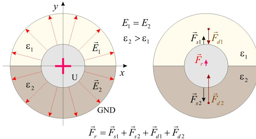
Figure 1: The cross section of the cylindrical capacitor filled with two different dielectrics, and force components.
