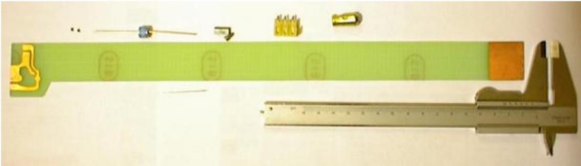
Figure 20: The etched PCB with sample parts.
