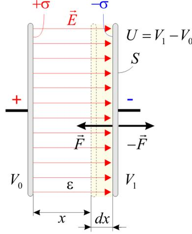
Figure 4: Deriving the equation of the electrostatic pressure from the law of energy conservation.
