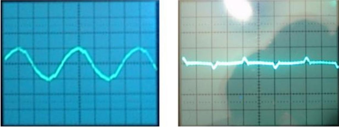
Figure 27: The parasitic 50 Hz signal with disconnected HV probe tip (left); and the same measurement when the output is filtered with a parallel capacitor (right); (0.2 V/div; 5 ms/div).
