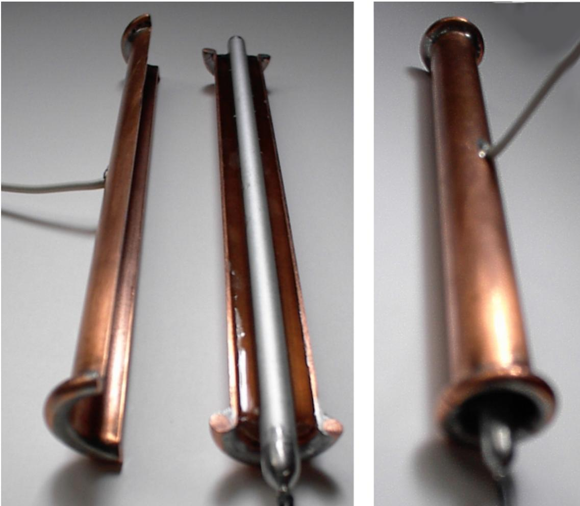
Figure 9: The finished 180° sector filled with polyester resin (left), and the assembled cylindrical capacitor (right).
