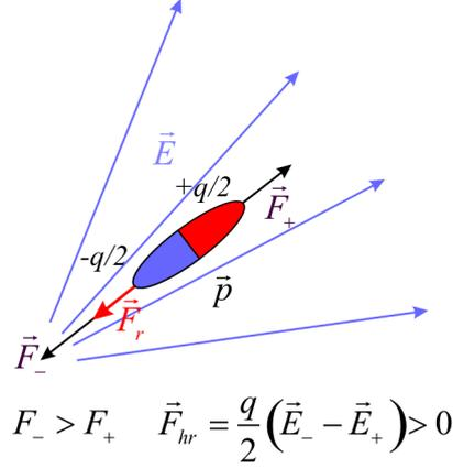
Figure 11: A possible modified model of the dielectrophoretic force upon an elementary dipole.
