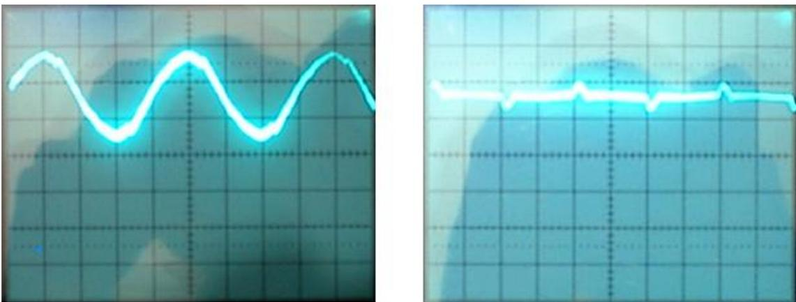
Figure 28: The unfiltered and the filtered output signal shapes of the probe when measuring the 320 V DC on the rectifier (0.2 V/div; 5 ms/div).
