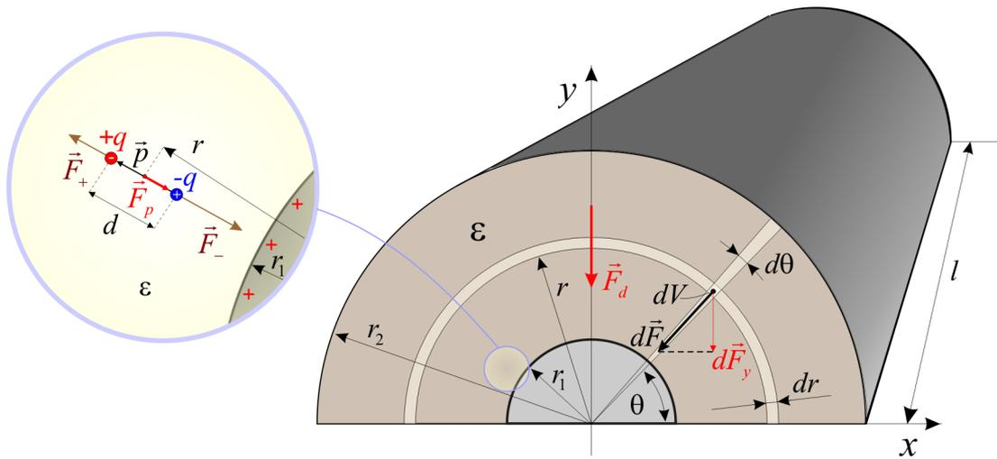
Figure 3: Calculating the dielectrophoretic force component on the bulk of dielectric.
