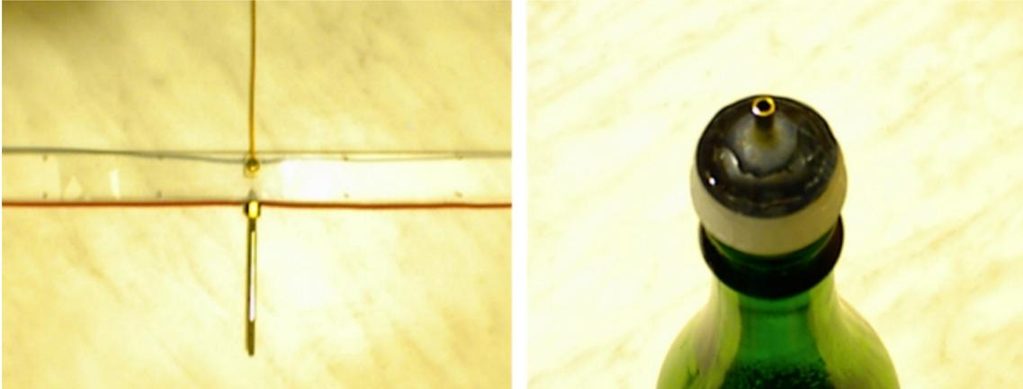
Figure 15: The ground- and HV wires mounted on the beam (left), and the HV contact 'bearing' (right).
