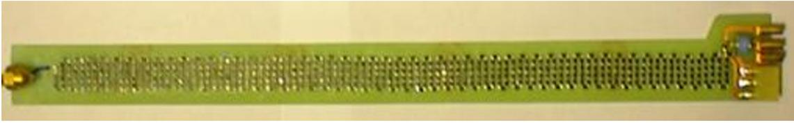
Figure 21: The PCB with mounted parts and soldered resistor-chain.
