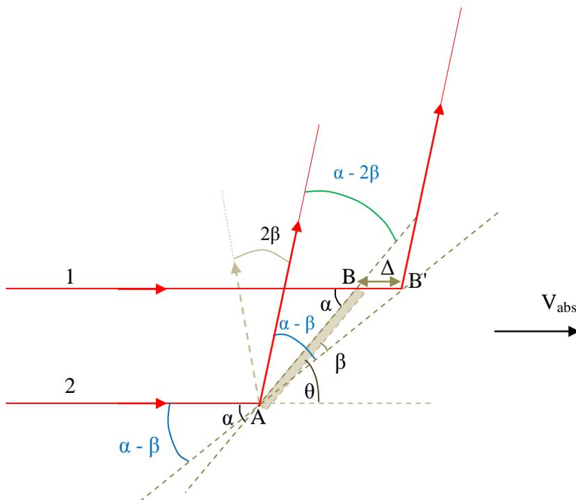
Therefore, the effective angle of incidence is  $\alpha - \beta$ . The angle of reflection should also be  $\alpha - \beta$ . Relative to the actual mirror (in the reference frame of the mirror), the angle of incidence is  $90^\circ - \alpha$  and the angle of reflection is  $90^\circ - (\alpha - 2\beta)$ ! The reflected light ray will be inclined forward by angle  $2\beta$  relative to the reflected ray in the case of zero absolute velocity.
