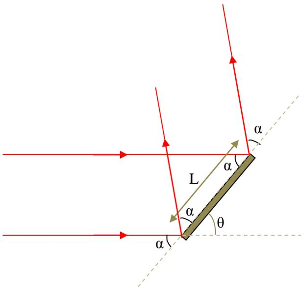
Next consider light reflection from a mirror that is moving to the right with velocity  $V_{\text{abs}}$  in the ether.
