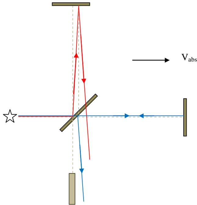
We can see from the above diagram that, even in the reference frame of the MMX apparatus, the transverse light beam ( red line ) will be bent forward on reflection from the beam splitter due to motion of the apparatus relative to the ether and there would be no interference pattern because the two light beams will not meet at the point of detection. The transverse light beam will miss the detector.
