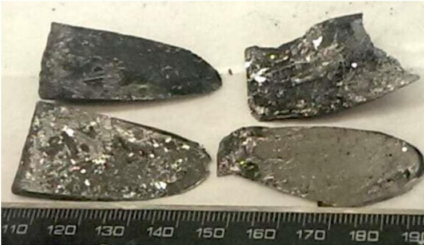
These single crystals of nickel-doped compounds of sodium, iron and arsenic are like those used by Rice University researchers in experiments to determine the material's superconductive properties at ultracold temperatures. They used [...more](#)
