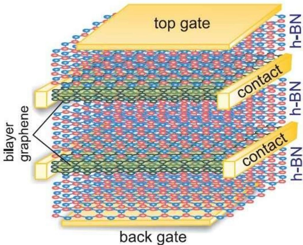
Device schematic: one sheet of conductive bilayer graphene carries electrons, the other, separated by insulating hBN, carries holes. Credit: FLEET
