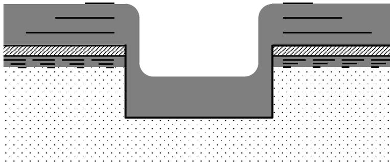
Step 7: Etch both sides down to the Ru layers.
