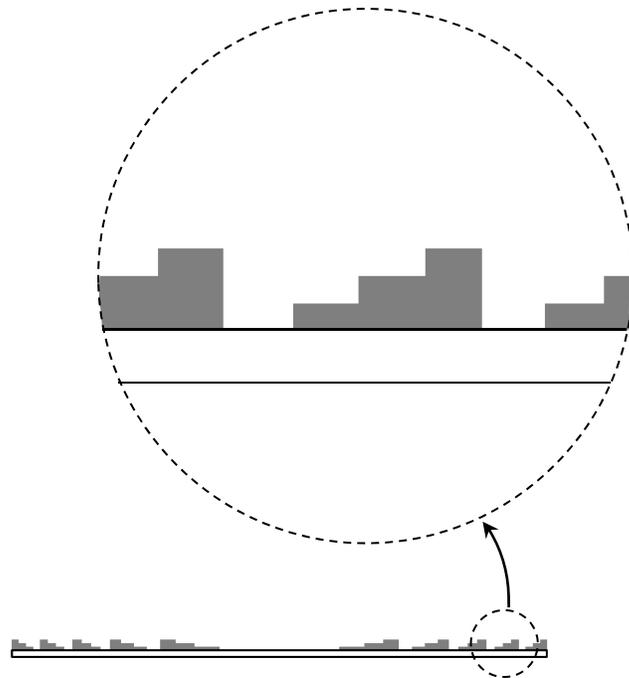
Figure 3. Cross-section of a stepped, 4-level phase-Fresnel lens.
