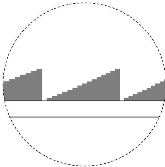
Figure 7. Single-sided EUV lens with 15 layers.
