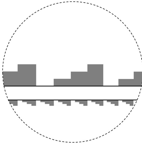
Figure 6. Double-sided EUV lens with 3 layers on each side.
