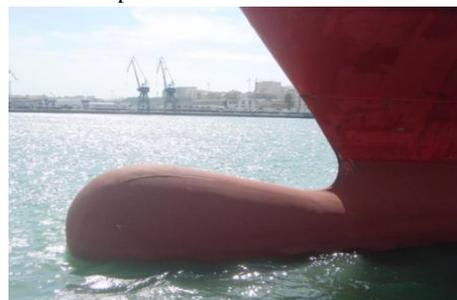
Fig. 17: Front bulb of a ship.
