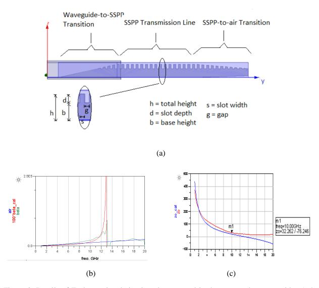
Figure 2. Details of E-plane printed circuit to be mounted in the rectangular waveguide. a) the side view; b) computed and simulated propagation constant as a function of frequency; and c) computed and simulated characteristic impedance of the SSPP line as a function of frequency.
