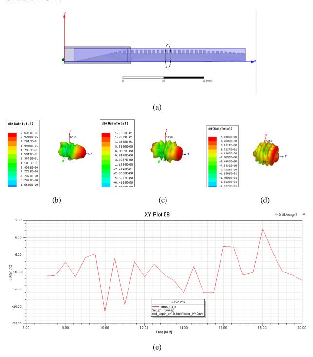
Figure 3. An E-Plane endfire antenna with linearly tapered SSPP-to-air transition. a) side view; b) Radiation Pattern at 8 GHz; c) Radiation Pattern at 9 GHz; d) Radiation Pattern at 10 GHz; and e) Simulated S-parameters.
