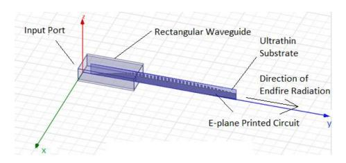
Figure 1. Basic version of the proposed E-plane endfire antenna.
