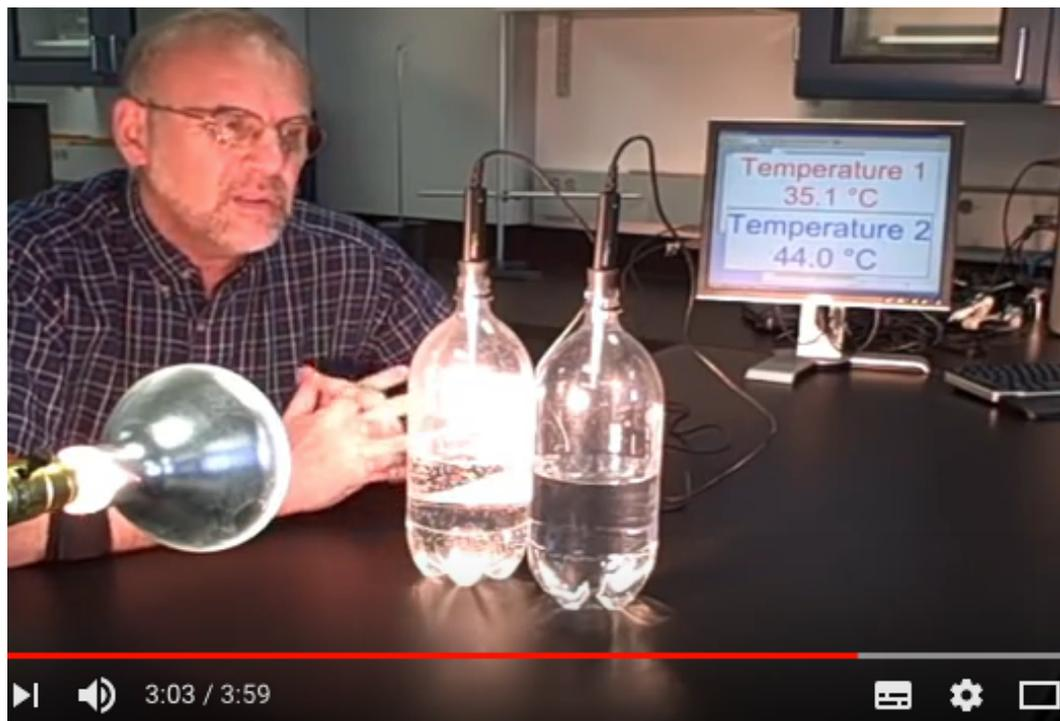
**Figure 39. Greenhouse Gas Bottle Demonstration [82].** Bottles with CO<sub>2</sub> and air are radiated and temperature measured – CO<sub>2</sub> in blue. Is this not an experiment to measure the heat capacities of the respective gases?
