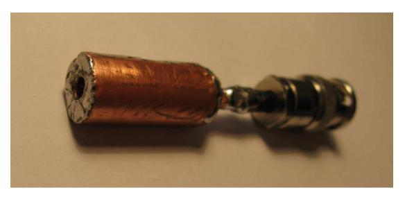
Micro scalar gun: external diameter is 13mm, hole = 4mm, legth (head) is about 30mm. The micro scalar gun is connected as pictured to the pulse generator:
