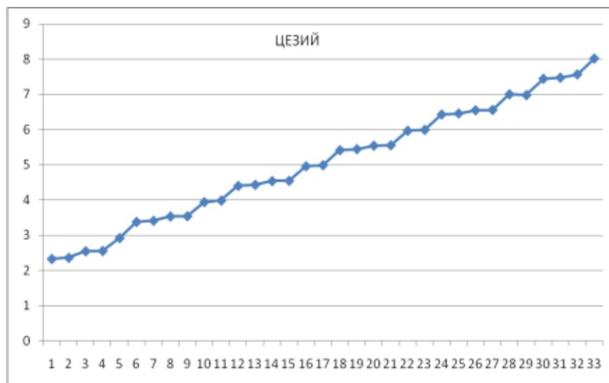
Fig. 14. Spectrum  $n$  of excited states of cesium atom.
