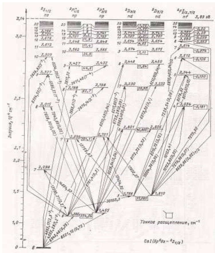
Fig. 13. Grotrian diagram of cesium atom [2].
