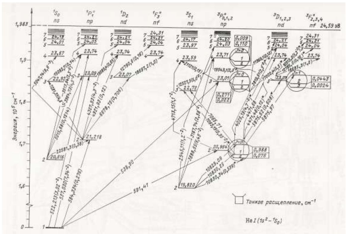
Fig. 5. Grotrian diagram of helium atom [2].
