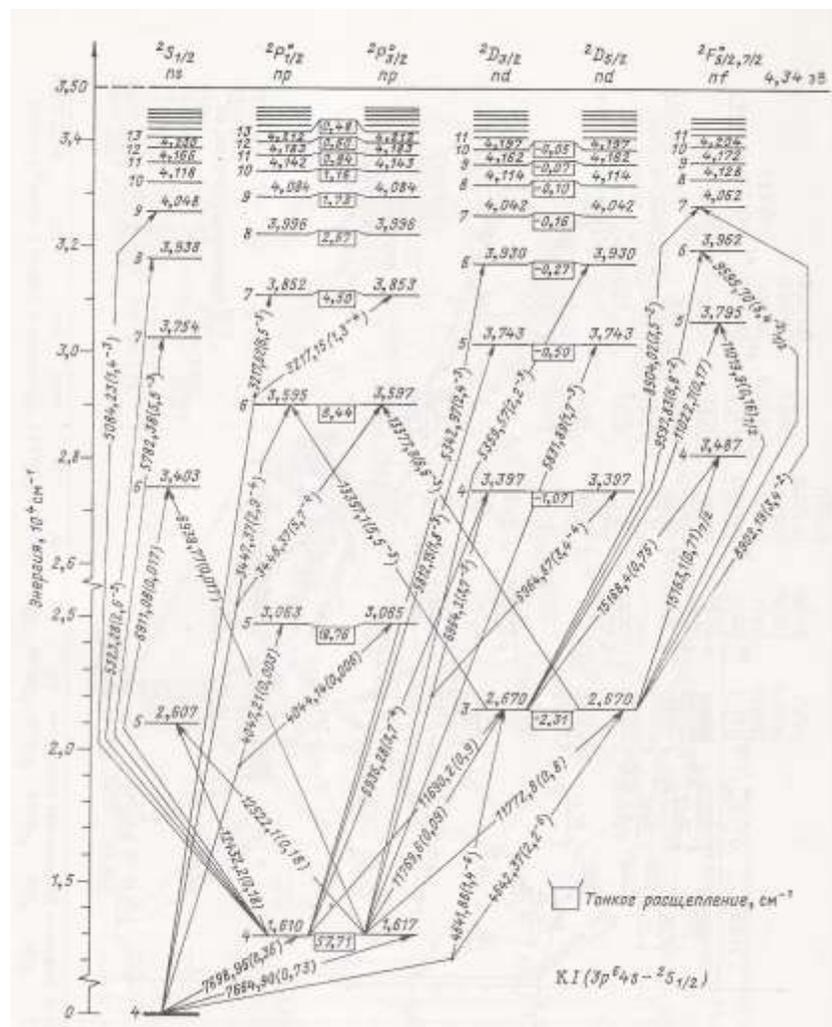
Fig. 11. Grotrian diagram of potassium atom [2].
