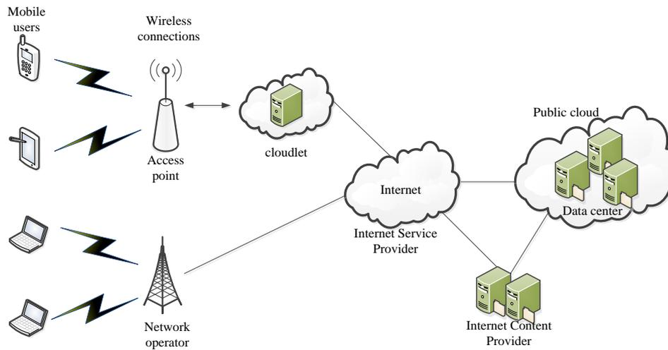
Figure 1 Architecture of Mobile Cloud Computing
