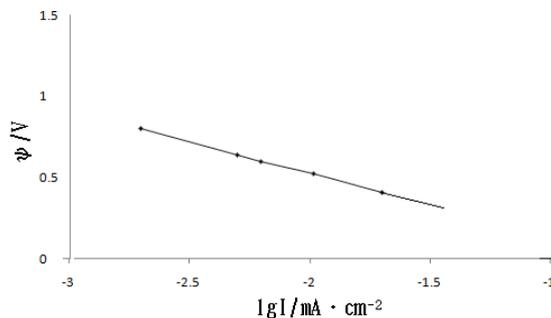
Fig.2 Cathodic polarization curve of electrolytic process
