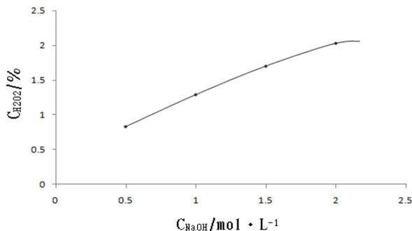
Fig. 4 Concentration change of hydrogen peroxide increasing with concentration of sodium hydroxide
