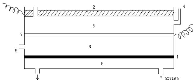
Fig.1 Schematic of device for preparation of hydroxide peroxide.
