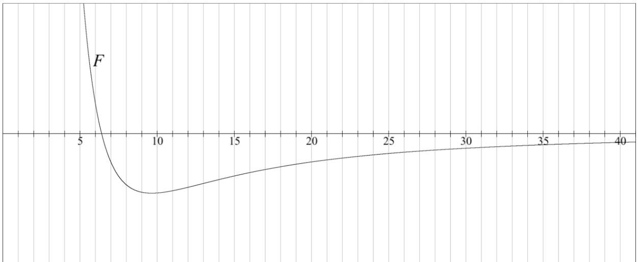
Fig. 4.0.1b. Detail: total gravitational force of the tensegrity icosahedron
