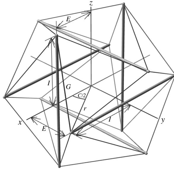
Fig. 2.1.1. Tensegrity icosahedron with Cartesian axes
