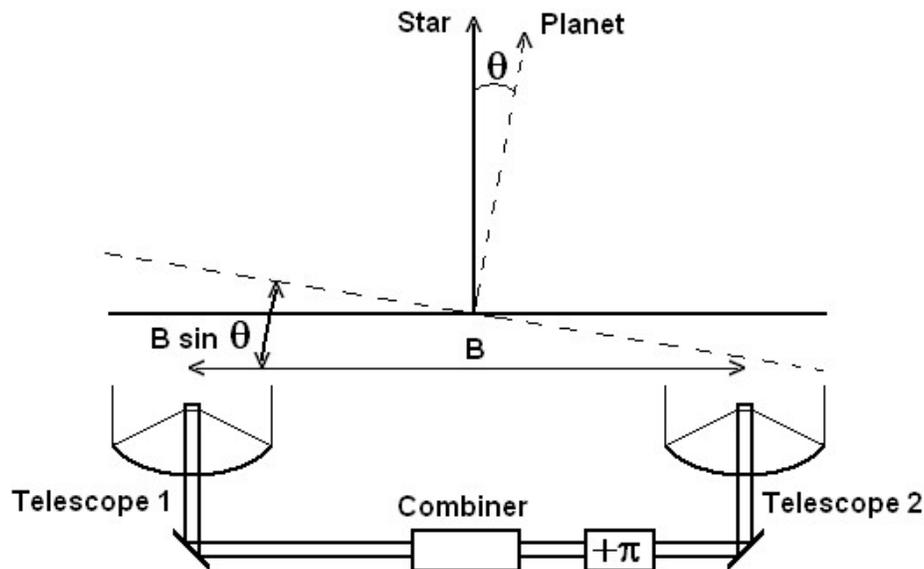
**Figure 1.** Two telescope space-based nulling interferometer, simplest configuration for producing a dark fringe in the line of sight when properly phased. This destructive interference enables planet detection by subtracting stellar coronas when focusing the null region on the stars disk. Redrawn from [63].
