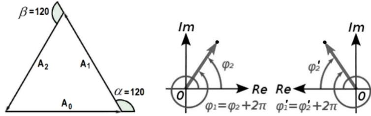
**Figure 1.** a) Phasor diagram of three waves in *perfect* destructive interference. b) Left-Right phase argument, preparation for phase transition channels in Dirac-Majorana duality modes.
