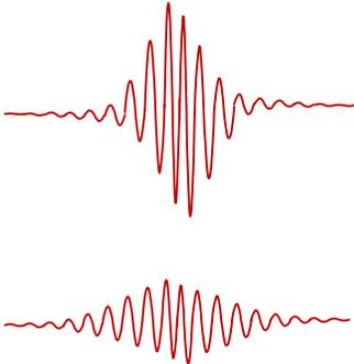
The next figure shows two photons of equal peak amplitude ( equal envelop peaks). The photon with higher frequency will be more localized than the photon with lower frequency.
