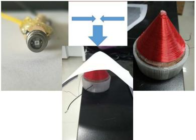
Fig 3: The configuration of TFC on the transmitter side
