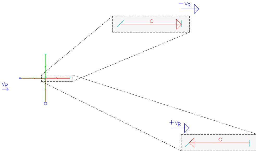
Fig. 18: Velocities on Michelson Morley experiment in dragged aether
