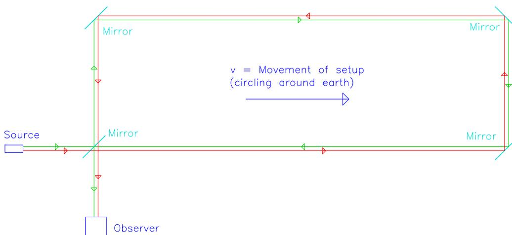
Fig. 15: Schematic setup of the Michelson/Gale/Pearson experiment
