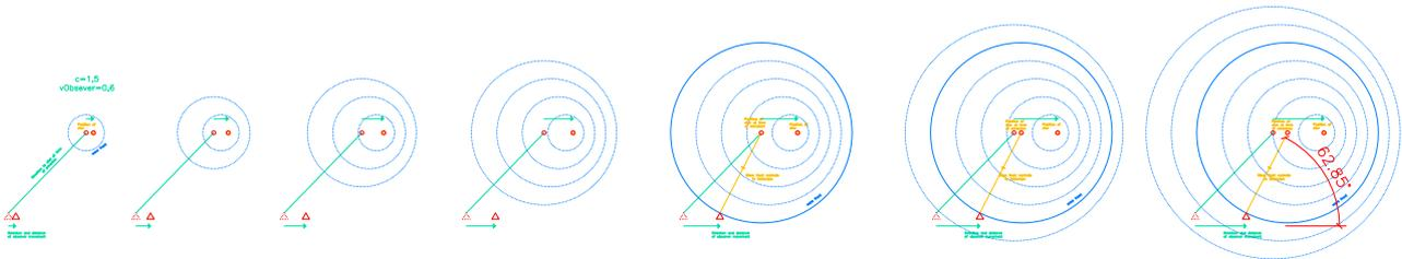
Fig. 7: Light propagation from source speed 0,6 km/s with 0,3 seconds steps, earth's speed 0,6 km/s
