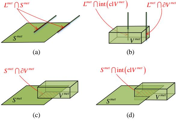
Fig. 2. (a) A part of metallic line contacts with metallic surface, and this case is not considered in this paper; (b) a part of metallic line contacts with or is submerged into metallic body, and this case is not considered in this paper; (c) a part of metallic surface contacts with metallic body, and this case is not considered in this paper; (d) a part of metallic surface is submerged into metallic body, and this case is not considered in this paper.
