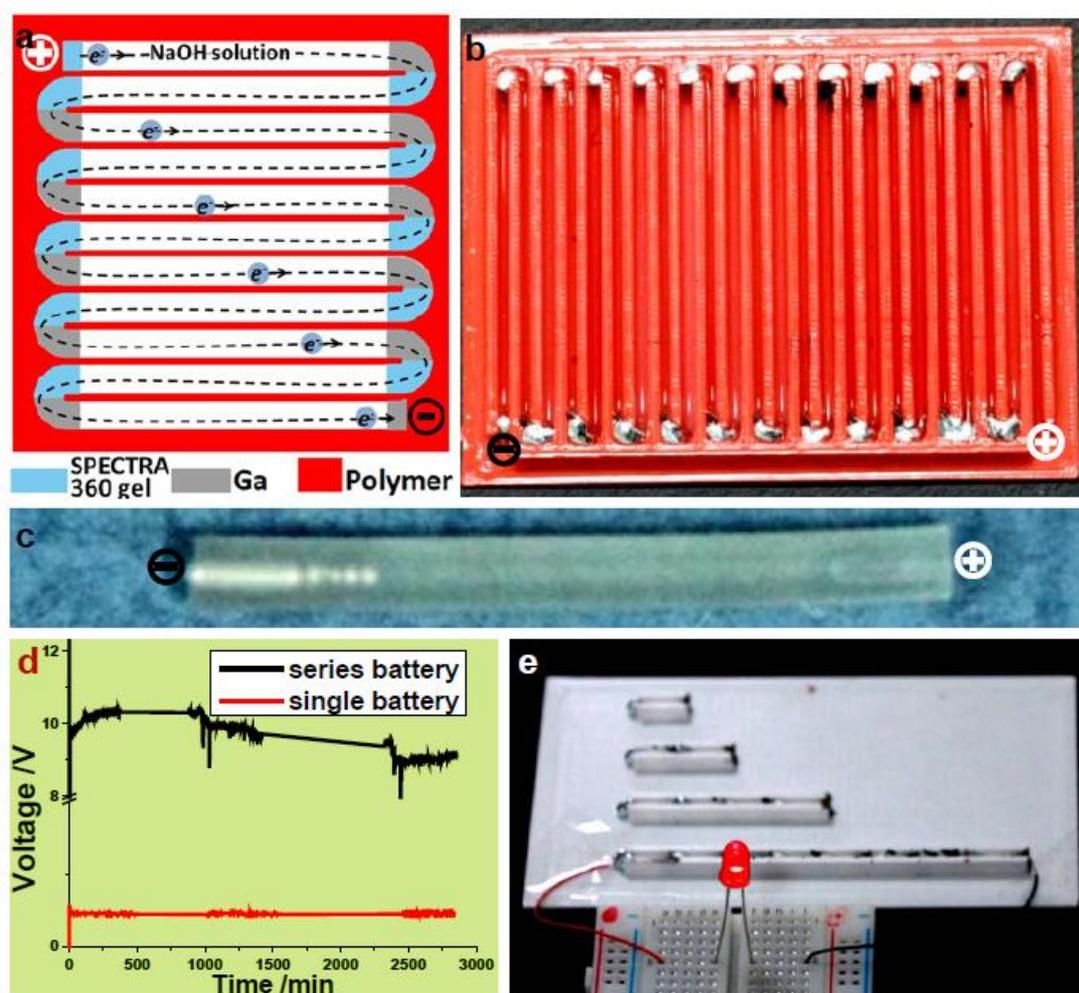
**Fig. 2.** Electrochemical study of liquid metal batteries. a) presents the schematic for battery with multiple cells, where the dotted line indicates the migration of electrons inside batteries during charging process; b) and c) present images of liquid metal batteries of 24-cell series and single one, respectively; d) presents discharge curves of
