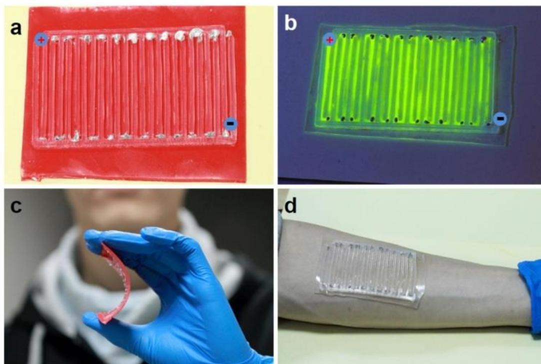
**Fig. 6.** a) Flexible battery was fabricated by TPU on 3M soft double-sided tape; b) Rhodamine solution was used to fulfill the cells and the picture was taken under UV lamp to clearly show the structure of cell body; c) Fabricated battery was flexible and can be twisted in any shape; d) Flexible liquid metal battery on skin: after removed the red substratum, the flexible and transparent battery can be bonded anywhere on the skin, according to applications.
