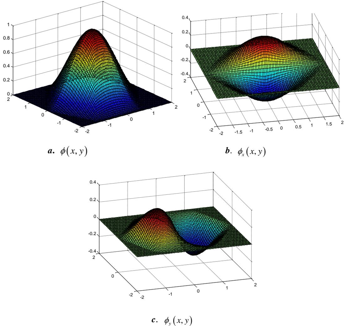
**Fig.3.**The basic full node shape functions  $\phi(x, y)$ ,  $\phi_x(x, y)$ ,  $\phi_y(x, y)$  at the coordinate origin
