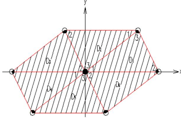
**Fig 2.** The extended hexagon domain enclosing a node at the coordinate origin
