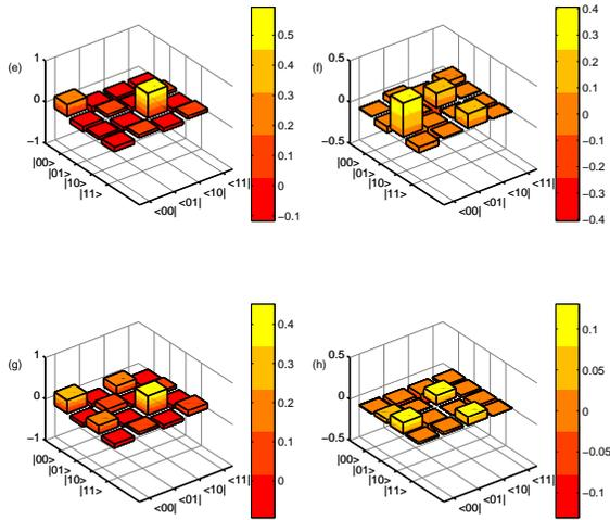
FIG. 6: (e) and (f) are theoretically predicted real and imaginary part of density matrix elements after four time steps of evolution with a double-well potential; (g) and (h) are the experimentally reconstructed density matrix elements after the four time steps in our two qubit-system.
