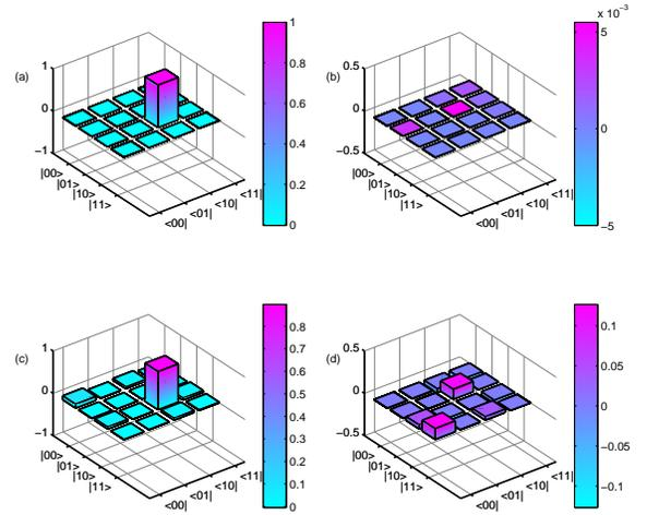
FIG. 5: (a) & (b) are the theoretical real and imaginary parts of the density matrix elements of the  $|10\rangle$  state; (c) and (d) are the experimentally reconstructed density matrix elements for the initial  $|10\rangle$  state in our two-qubit system.
