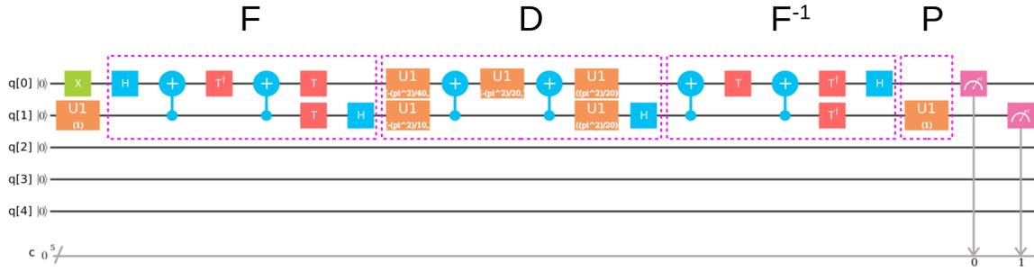
FIG. 1: The two-qubit quantum circuit for one time step simulation. The quantum circuits for the kinetic ( $FDF^{-1}$ ) and potential (P) energy operators are depicted.
