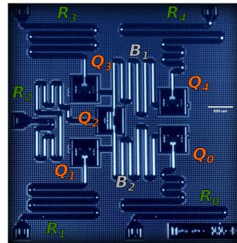
FIG. 2: Two coplanar waveguide (CPW) resonators provide the connectivity between the 5 transmon qubits. For the control and readout of the qubits, a CPW is associated with each qubit.
