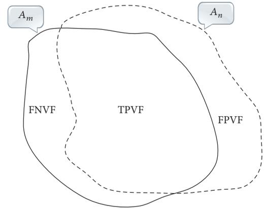
FIGURE 8: The areas corresponding to TPVF, FPVF, and FNVF, respectively.  $A_m$  indicates the “true” contour delineated by the radiologist and  $A_n$  denotes the contour obtained by the segmentation algorithm.
