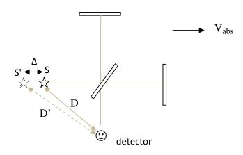
From the above diagram of the Michelson-Morley experiment, we see that the effect of absolute velocity is just to create an *apparent* change of the position of the light source *relative* to the detector. The apparent change in position is determined by the direct source-detector distance D, the orientation of the source-detector line with respect to the absolute velocity and the magnitude of the absolute velocity[1].
