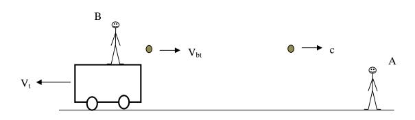
Therefore, the velocity of the balls relative to observer A is constant c independent of the velocity of the truck, analogous to the speed of light being constant c relative to an observer at absolute rest, independent of source velocity.
