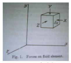
Fig. 1 – Forces on fluid element.
