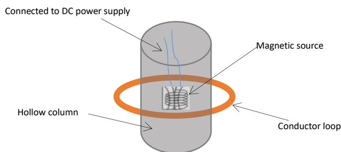
**Fig.2.** A magnetic source is located in the middle of a conductor loop. The magnetic Source is surrounded by a hollow column made of magnetic shielding material
