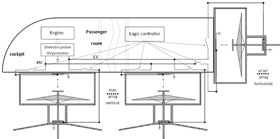
Array deployment can optimize the entire geometry configuration, for example, if 10 square meter umbrella area is required, then for single umbrella solution, the umbrella height could be 2 meters, in contrast, if 10 umbrellas array with 1 square meter each, then it can better match the chassis shape, e.g. in  $2 \times 5$  array, and the height could be about only 0.6 meters.
