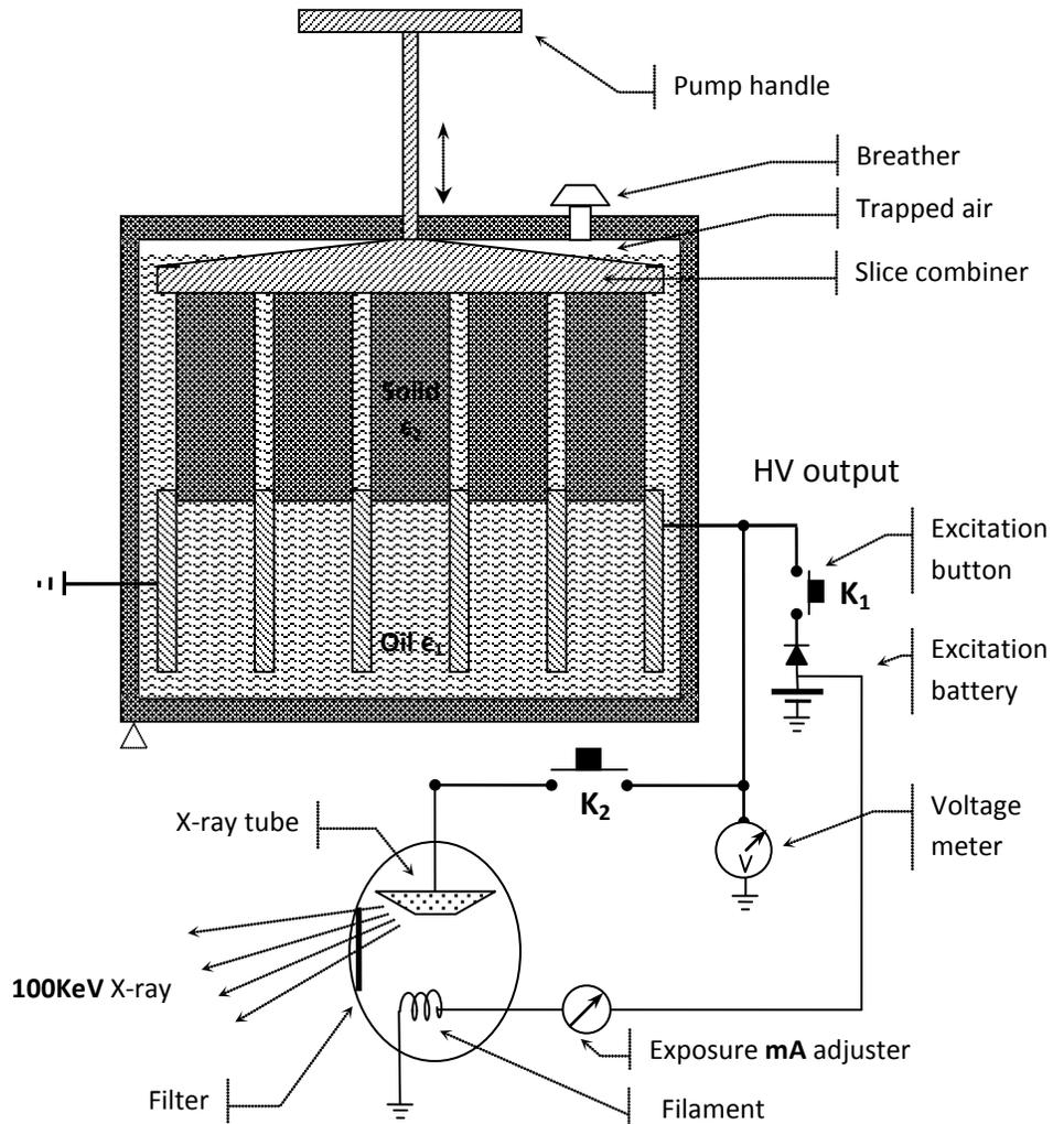
Fig. 10: simple hand pumped hydraulic mobile pulse X-ray source
