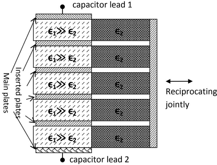
a. cascade mode, total capacitance = embedded\_capacitance/( $N+1$ )
