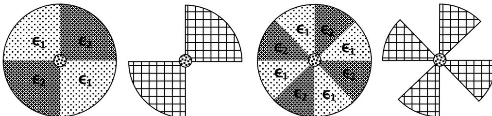
Electrode plates area = 50% of disc area for many applications
