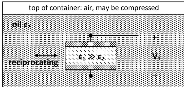
**Fig. 1:** dielectric media reciprocating displaceable capacitor voltage transformer
