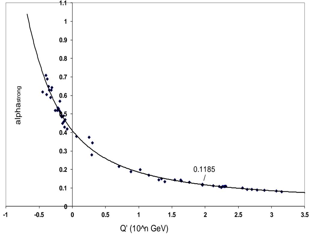
Figure 2. The theoretical variation of  $\alpha_s$  with momentum transfer, as calculated from Eq.(3.1), which gives  $\alpha_s(M_{Z_0}) = 0.11854$ . Empirically,  $\alpha_s(M_{Z_0}) = 0.1185 \pm 0.0010$ . Data points have been taken from Bethke (2007) Table 1, and Baldicchi et al (2007) Tables 1-7 for  $Q > 150\text{MeV}$ , and CMS Collaboration (2015).
