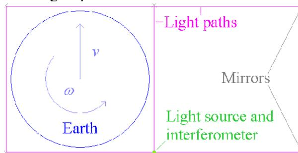
**Figure 13.** In this ether drag experiment, the light source sends beams along all violet light paths, which are created by mirrors at the square corners. An interferometer reads the fringes of recombined returning beams. The left square measures ether drag due to Earth’s rotation, while the right measures ether drag due to translation.
