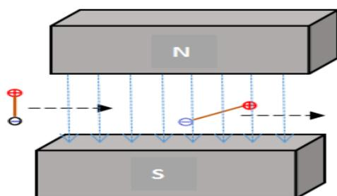
**Fig. 1.** An electric dipole moving across a magnetic field
