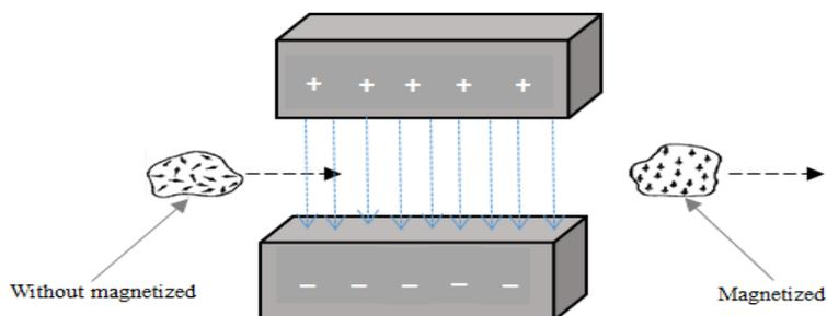
**Fig. 3.** A bulk of magnetizable material moving across an electric field
