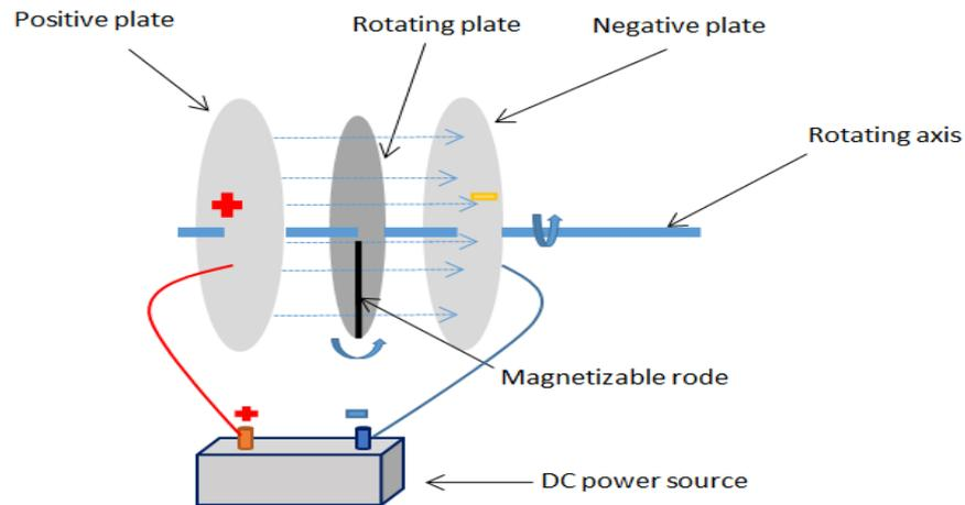
**Fig. 4.** Experimental design to verify the existence of this force
