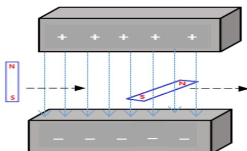
**Fig. 2.** A magnet moving across an electric field
