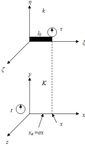
Fig. 2: Two systems of clock-synchronised stationary observers that are at rest. The system  $k$  contains a rigid rod of length  $\xi = l_0$ . All observers agree as to its length at any time.
