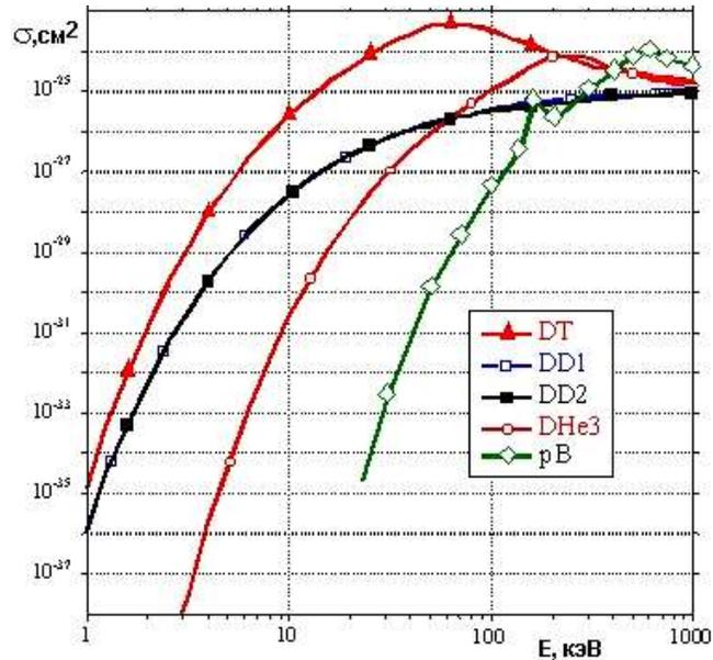
**Fig.1.** Thermonuclear cross section reaction of D+T, D+D (1), D+D (2), D+<sup>3</sup>He, and p+B vs kinetic energy E [Kev] of the particles.
