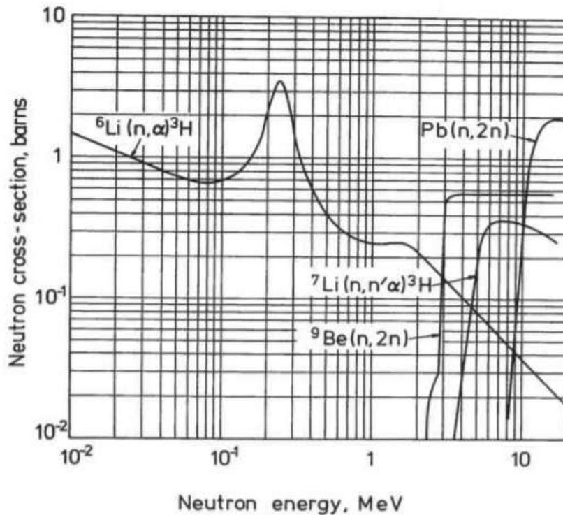
**Fig.2.** Cross section for reaction  ${}^6\text{Li}(n,\alpha){}^3\text{H}$ ,  ${}^7\text{Li}(n,n'\alpha){}^3\text{H}$ ,  ${}^9\text{Be}(n,2n)$ ,  $\text{Pb}(n,2n)$ . Other important cross sections include elastic and inelastic scattering cross sections for Li, Be, Pb, needed for the slowing down (moderation) of the 14 MeV primary neutrons and neutron absorption cross sections for structural material (Figure from M. Sawan).
