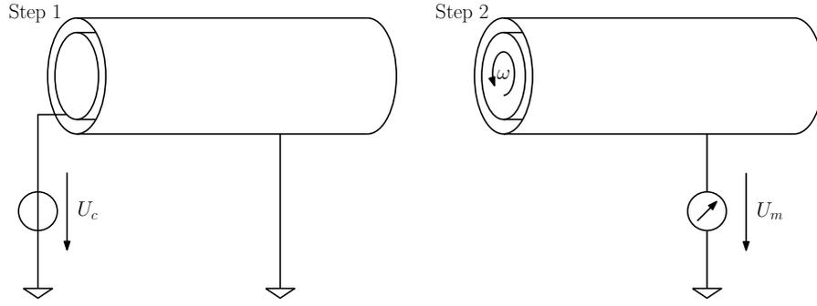
Figure 1: A cylinder capacitor is charged and then decoupled from voltage source and ground. In the second step, the inner cylinder is brought into rotation.
