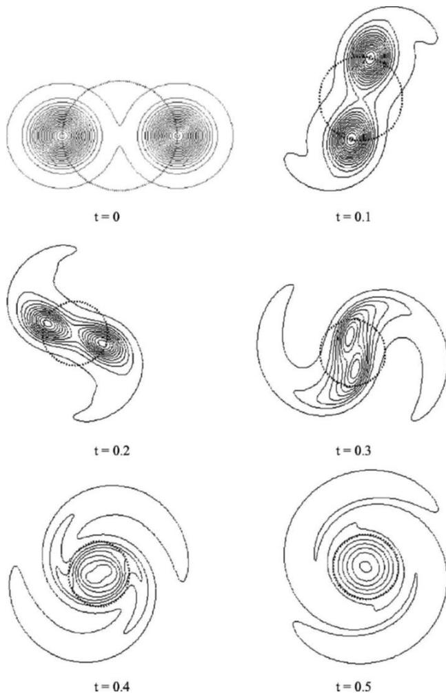
Fig. 4. Time evolution of the vorticity contours during the merging process of two equal co-rotating vortices with equal angular velocities. A circle with constant diameter is plotted for reference. Figure from Huang's article above mentioned, used by permission.
