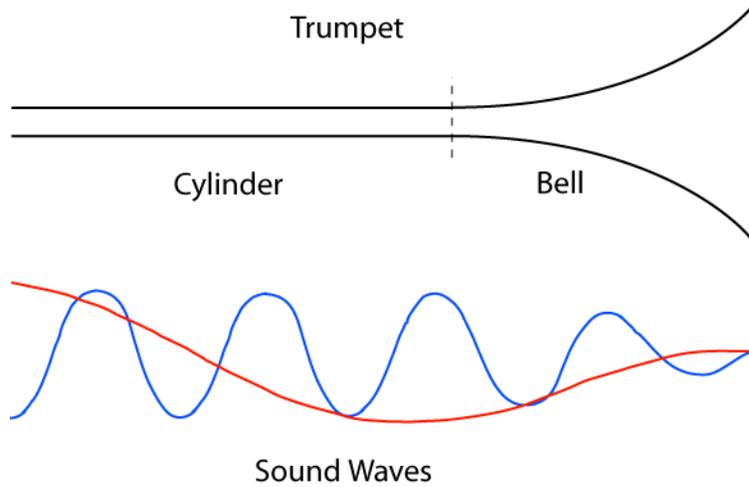
**Figure 21.** Standing waves in a trumpet
