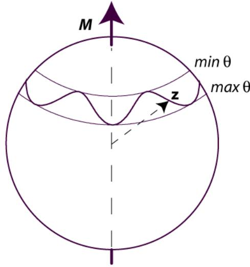
**Figure 9.** The trajectory of the spin vector  $\mathbf{s}$ .
