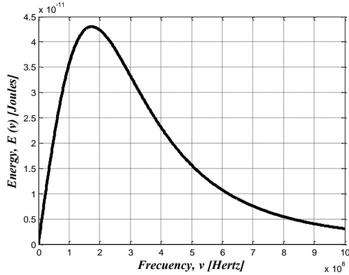
Figure.3. Energy spectral distribution radiated by the *Hertz* dipole.
