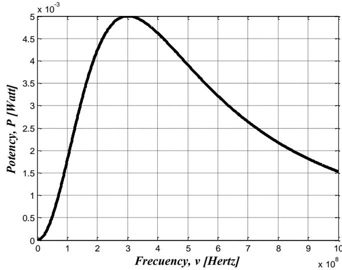
Figure.2. Power spectral distribution radiated by the *Hertz* dipole.
