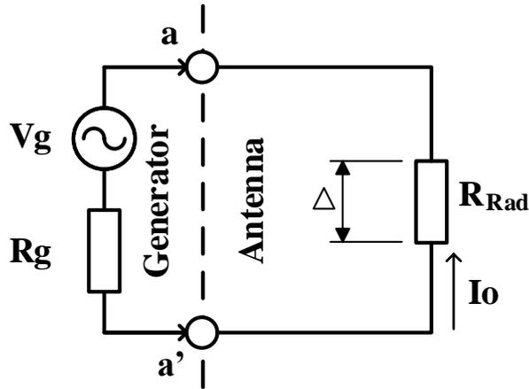
Figure. 1. Antenna-generator system.
