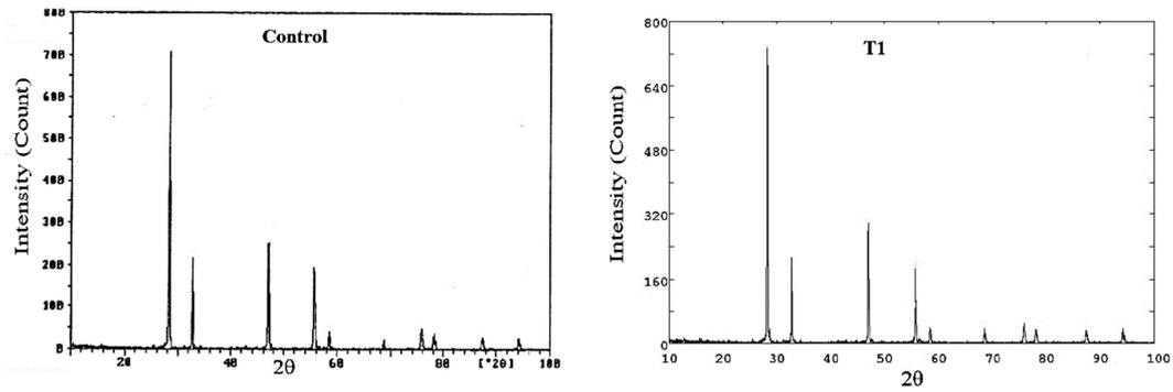
Fig. 3. X-ray diffractogram of praseodymium oxide powder.
