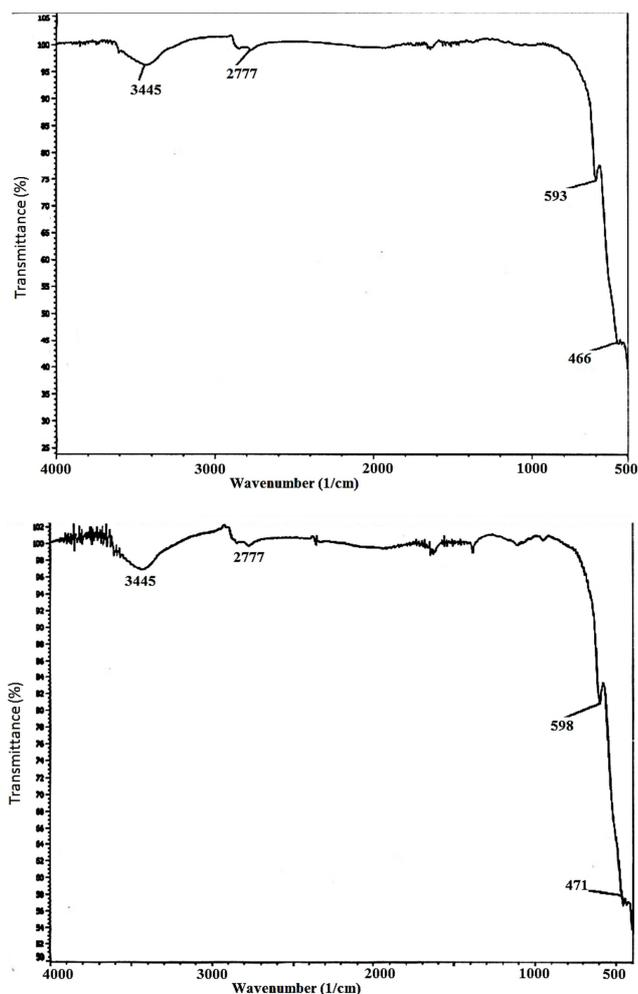
Fig. 5. FT-IR spectra of praseodymium oxide powder.
