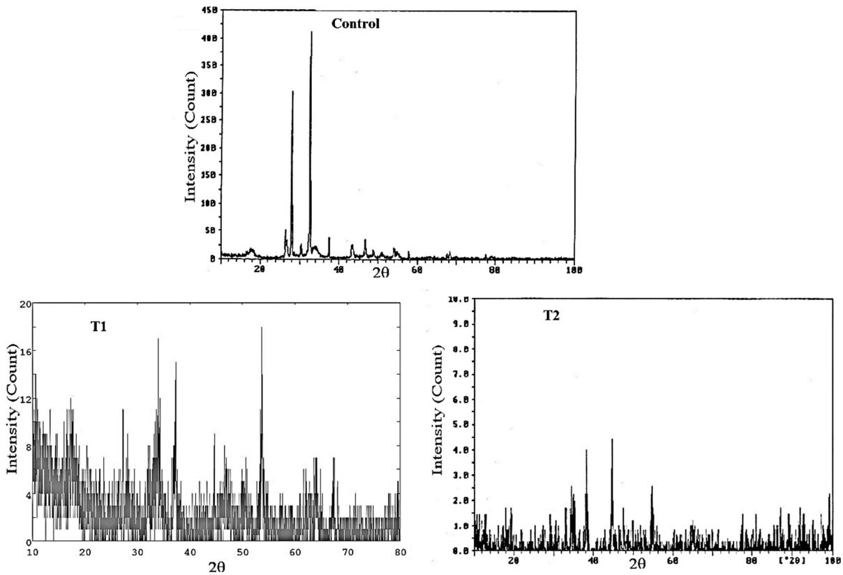
Fig. 1. X-ray diffractogram of calcium carbide powder.
